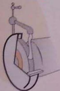
*In case of using coolant, turn off coolant from 2 up 10 minutes stopping wheel to avoid creating an out of balance condition.*
